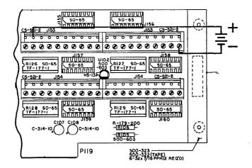
Figure 2. Typical AIM3 Single-ended Connections (Channel 0 shown)
