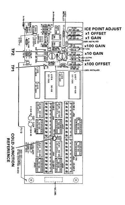
Figure 4. AIM3 Calibration Adjustmets
